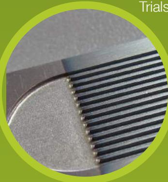
Trials are underway with alumina-coated stainless steel micro-reactors. The coatings are very thin, at approximately 100 nm.
