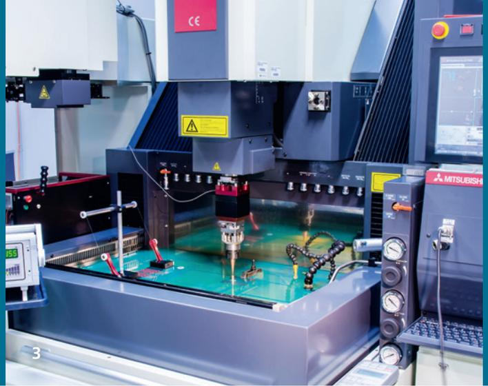
Numerous tests pointed out that high frequent vibrations on the electrode in z-axis direction causes current flows in the discharge gap, so material debris can be washed away. This finally leads to a consistent EDM process, whereby machining time will be reduced significantly by partly less electrode wear. Microvibe300 is not restricted to micro machining and can be successfully used for sinking processes with discharge currents up to 30 A and electrode weights up to 0.7 kg (incl. holder).
