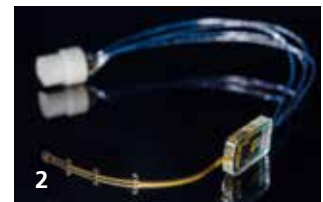
1 Detail of spinal electrode array | 2 Spinal electrode array with interface and electric connector
