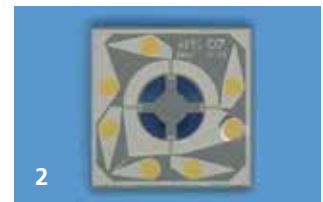
1 Piezo-resistive three-axial force transducer | 2 Sensor backside with piezo resistors and bond pads
