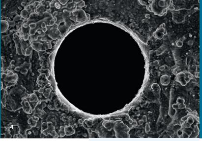
The combination of rotation and vibration in one unit additionally increases the precision of the machined hole, such as roundness, and improves the uniformity of the electrode wear.
