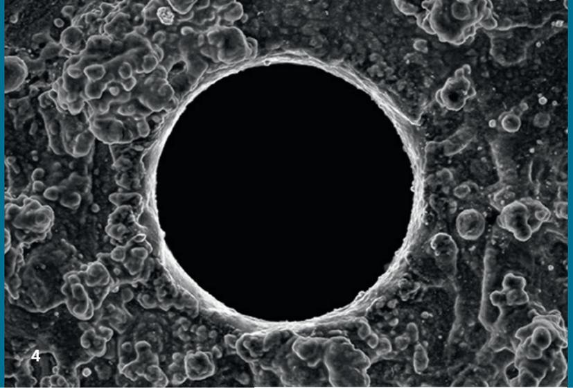
The combination of rotation and vibration in one unit additionally increases the precision of the machined hole, such as roundness, and improves the uniformity of the electrode wear.
