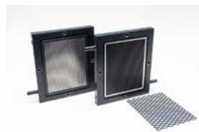
ShaPID reactor for formate synthesis from \text{CO}_2
