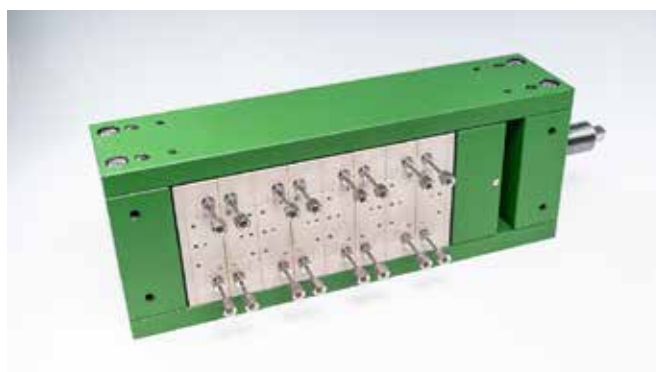
ELMISCREEN reactor for catalyst screening
