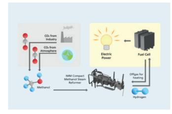
All these obstacles are overcome by innovative IMM self developed and patented catalyst technology, which follows a completely different route of the reforming reaction [1], [2]. Its stability and robustness has been proven in the lab by excessive long term testing and in practical operation in reactors of up to 35 kW scale. Since its invention a decade ago, the catalyst was continously improved.
