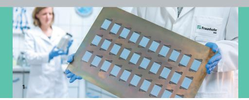
1 Stainless steel sheet with an array of 30 reaction plates coated with catalyst layer.
