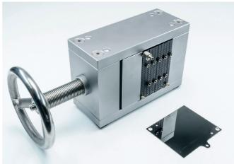
Typically, the core plates of the stack represent on both sides structured electrodes and are equipped with an integrated heat exchanger. These are realized by a combination of additive manufacturing to obtain the basic plates with their complex fluid structures, surface coating (e.g. with PTFE) of the basic plates for electric insulation, milling to create the micro channels on the plates surface and electroplating to deposit different electrode materials on the plates.
