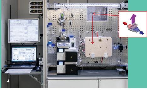
A key benefit of continuous syntheses is the tight process control and that the various process parameters such as flow rates and temperature can be adjusted to achieve the desired property, e.g. exciton wavelength in case of QDs. With our reactor, it is possible to tune the wavelength with sub-nanometer precision to the desired value in a stable process.
