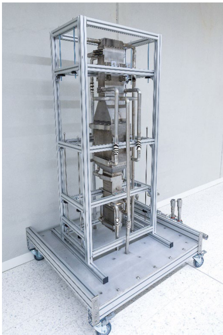
Fig. 1 Fraunhofer IMM pilot plant for ammonia cracking with ammonia cracking capacity of 20 kg/h
