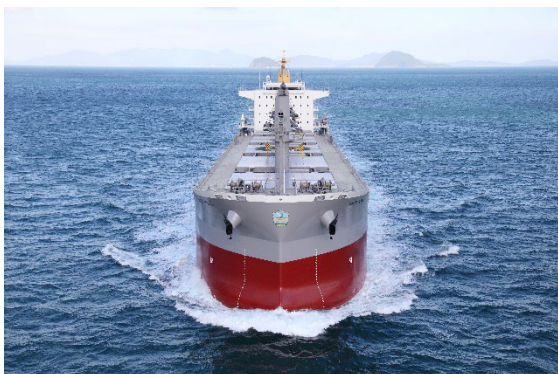
Fig. 2 As part of the EU's GAMMA project this freighter will be partially powered by an ammonia cracker from Fraunhofer IMM, which has an equivalent electrical output of 400 kW, together with a fuel cell.
