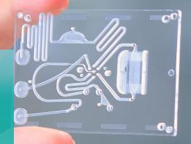
The use of microfluidics and the related system technology for the handling of liquid quantities from the micro- to picoliter range, the so called lab-on-a-chip technology, resulted in significant progress with respect to the development of efficient analysis methods.
