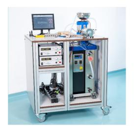
Mobile reactor unit for on-site use.
