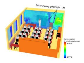
Numerical simulation of the aerosol dispersion within a classroom: An infected person sits in the front right corner of the classroom. The selected cross-section shows the concentration distribution of the virus-containing aerosol. A room air purifier filters the aerosol-laden air and returns it purified.
