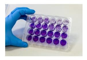
Fraunhofer researchers use virus infection tests, e.g. a plaque or TCID50 assay, to investigate whether the air still contains infectious and thus transmissible viruses after inactivation.
