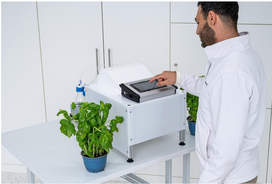
Figure: Test setup for the AutoNutri system in the Fraunhofer IMM laboratory. The test focuses on online process analysis technologies (PAT), which are used to improve quality control of water and nutrient solutions, as well as bioprocess streams. (© Fraunhofer IMM)
