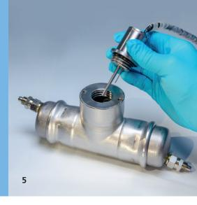
oil's current condition while it is operating. Main parts of the online sensor system are NIR-sensors, which detect contaminations (e.g. water, soot) as well as the total base number (TBN) through transmission- or ATR-cells and micromechanical sensors for viscosity measurement via shearing force (Fig. 5). Partners were developing particle-detecting-sensors.
