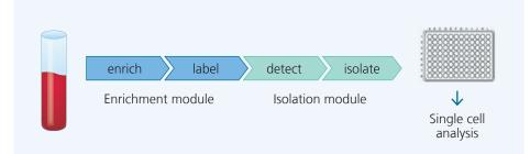
the CTCs, detects them in a continuous flow and dispenses single CTCs selectively into wells of a standard microtiter plate resembling the starting point for single cell analysis. The corresponding assay can be adapted by the user with an intuitive graphical user interface.
